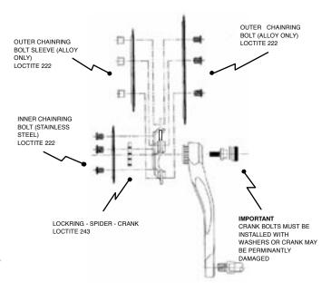
Apply loctite 222 locking compound (purple) to the chainring bolt threads and tighten alternately using a crossing pattern to eliminate un-even loading on bolts and avoid creaking. Torque to 100 lnLbs
